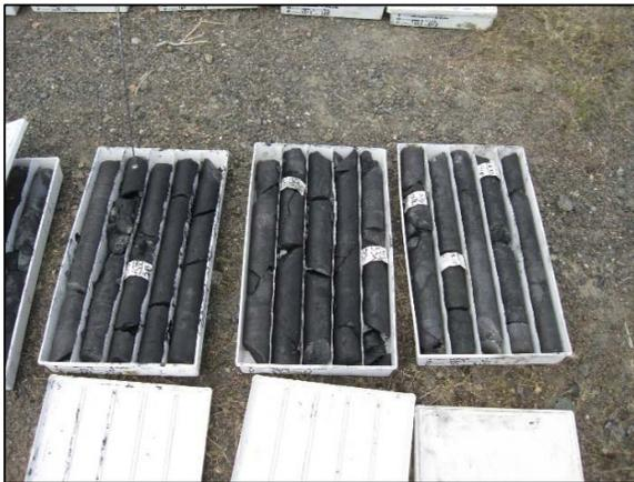
Figure 3: Massive magnetite in drill core
