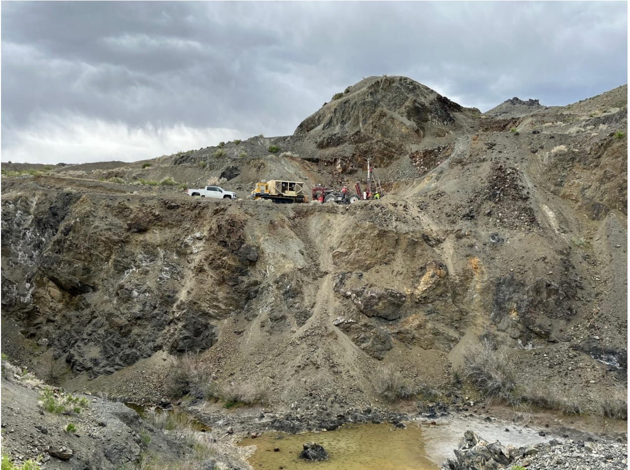
Figure 2 Drilling hole NF-06. Massive magnetite outcrop can be seen in the historic pit to the left of and above the drill rig.
