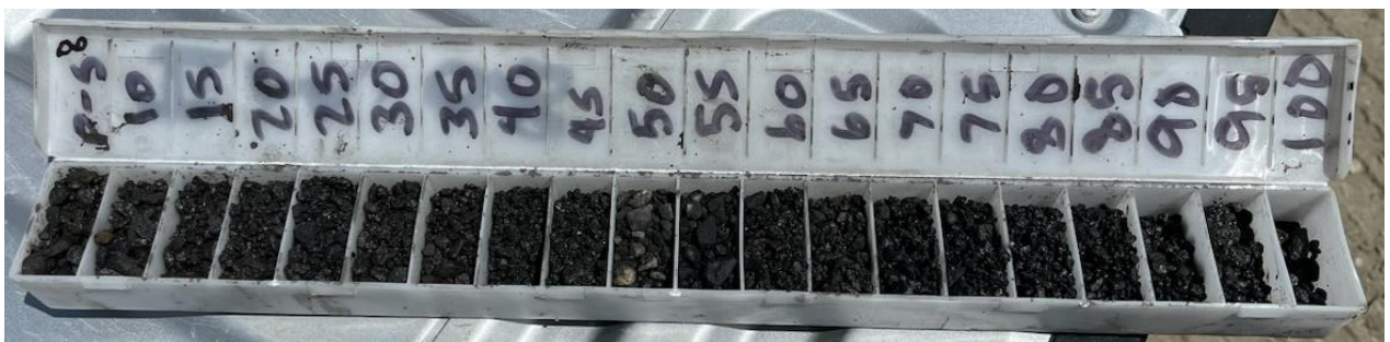
Figure 3 Thick intercepts of magnetite have been encountered. This is from RC hole IM-08. Note that depth labelling is in feet.
