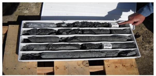
Figure 6: Drill cores showing metasomatic magnetite
