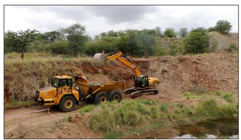
Photo 4: Blast material being loaded from the Cobra Pit
