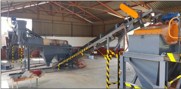
Photo 6: Plant dewatering screen with trommel and screen feed conveyor
