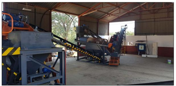
Photo 7: Plant crusher with oversize return conveyor and trommel
