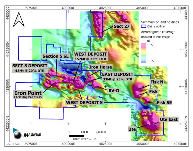
Figure 3 - Buena Vista Green Pig Iron Project: Image of recently collected aeromagnetic data showing resources and exploration prospect locations.
