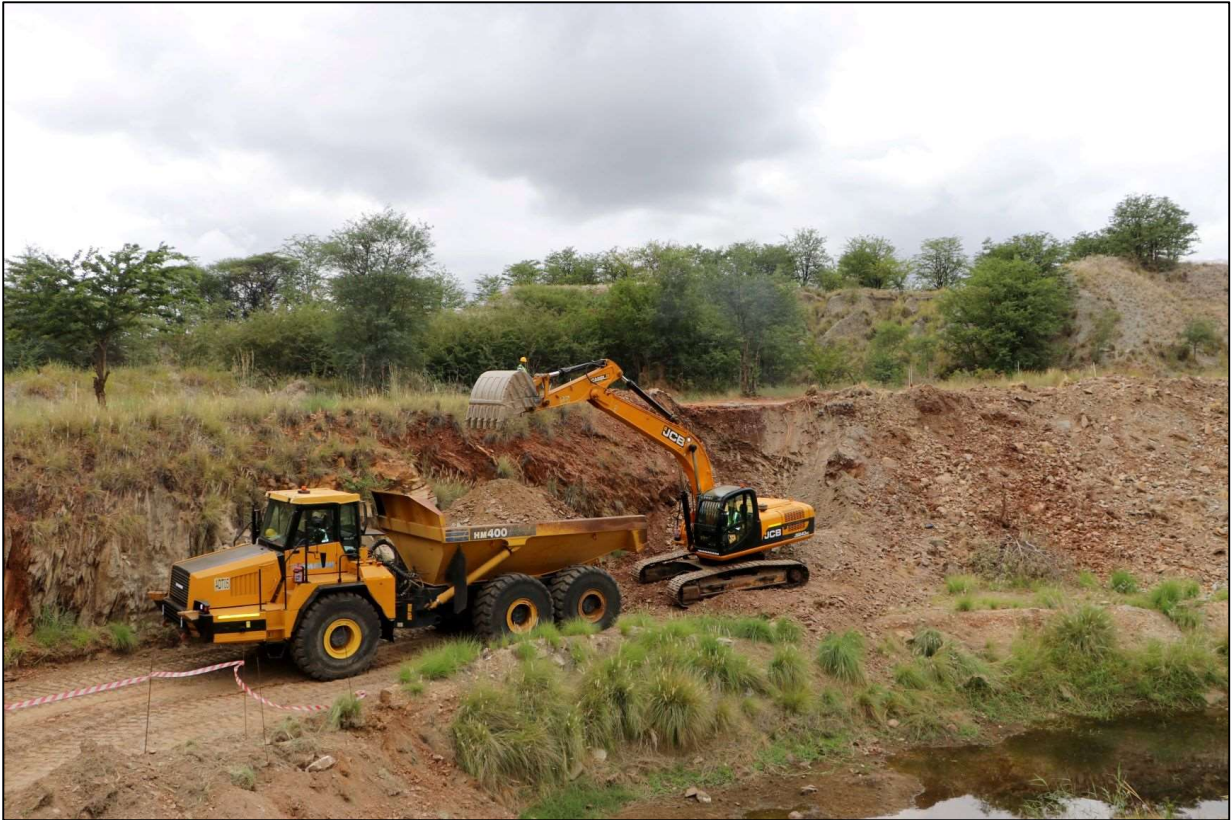
Photo 2: Cobra North Pit blast material being loaded
