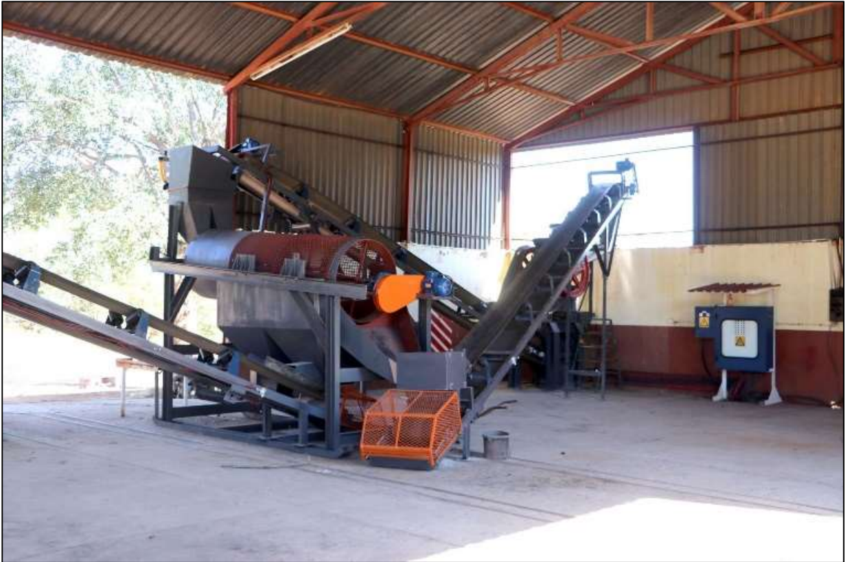
Photo 5: Plant crusher with oversize return conveyor and trommel
