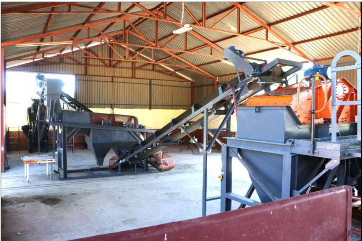
Photo 6: Plant dewatering screen with trommel and screen feed conveyor
