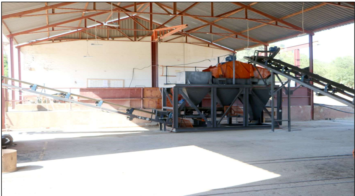
Photo 4: Dewatering screen and conveyor
