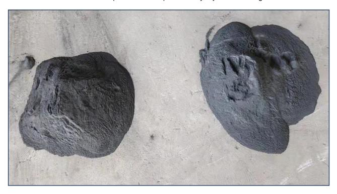
Figure 6: Buena Vista 63% magnetite iron ore concentrate.
