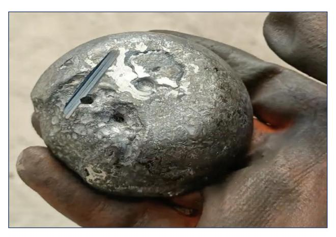
Figure 9: 100% biochar green pig iron using Buena Vista iron ore.
