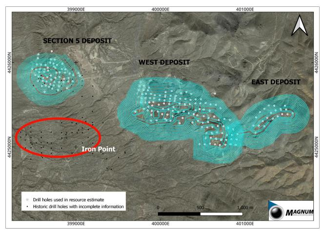
Figure 2: Iron Point Prospect area in the Buena Vista Green Pig Iron Project showing drill holes used in the MRE, other holes, and the proposed and conceptual pit locations and designs.
