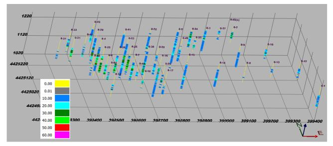
Figure 3: Summary of Iron Point Prospect drilling data used in the Exploration Target estimation. The grid is 100x100m (NAD83 Zone 11N).
