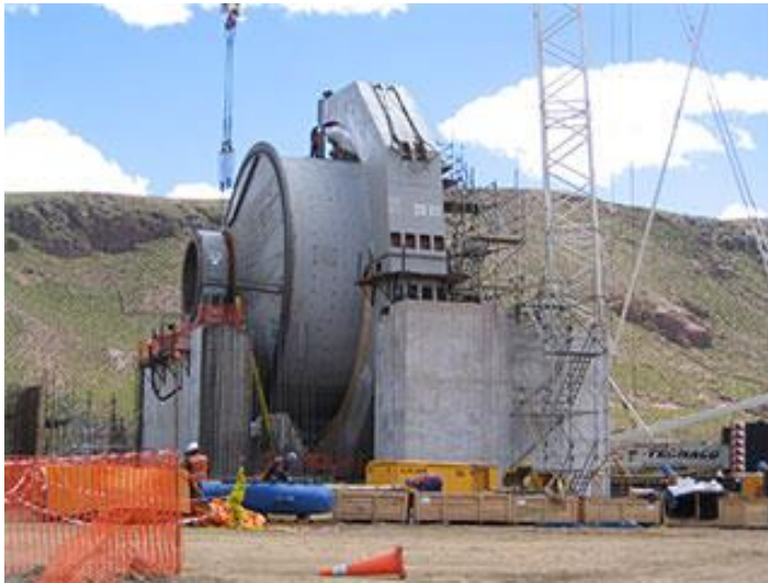
Figure 2 The Buena Vista Iron Project will utilise mills such as this one to grind magnetite ore to -63\mu\text{m} before magnetic separation. Illustrative purposes only.
