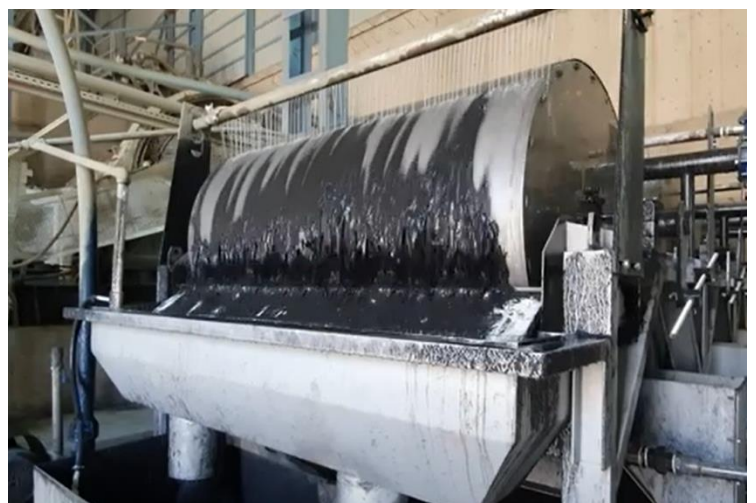
Figure 3 A Wet Low Intensity Magnetic Separator such as this is used to separate the magnetite grains from the gangue minerals (mainly silica). Illustrative purposes only.
