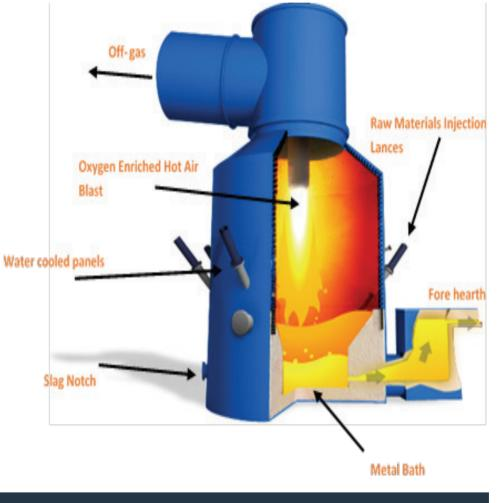
Smelt Reduction Vessel (SRV) at the Heart of Technology
