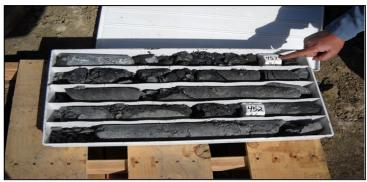
Figure 5: Drill cores showing metasomatic magnetite
