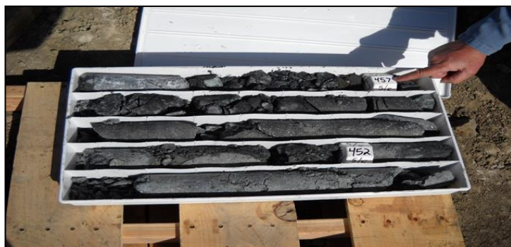
Figure 5: Drill cores showing metasomatic magnetite
