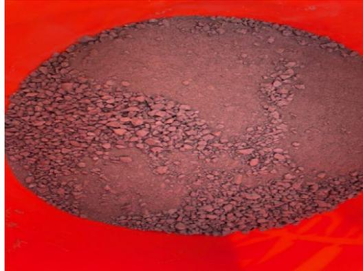
The sample was constructed to mimic the long run head grade based on the five-year mine schedule for the IMA. The Buena Vista Iron Project is based on a magnetite ore body that has had a successful Scoping Study completed in 2023. The magnetite ore can be concentrated using standard mining industry methods of crushing, grinding, and Low Intensity Magnetic Separation (LIMS).
