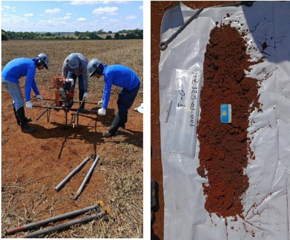
Figure 9 - Auger drilling to be undertaken by two three-man crews. Samples are to be collected at each 0.5m interval to a nominal depth of five metres at each site. Assaying will be done by ALS Laboratory, Brazil. 8
