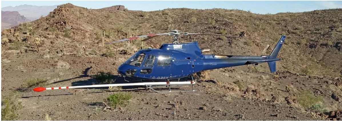
Figure 20 - Helicopter used for the ultra-high resolution airborne aeromagnetic and radiometric survey at the Parker Gold (Cu-Au) Project, shown at the base station magnetometer. 21
