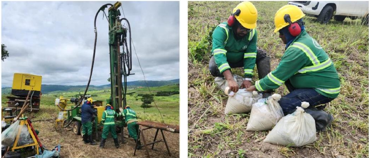
Figure 13 – Left: RC drilling on the Palmares REE Project, at the Feirinha Prospect. Right: Field technicians preparing RC drill samples from Feirinha. 11
