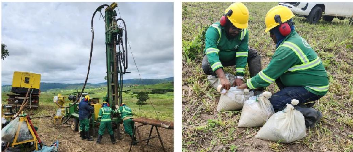
Figure 4 – Left: RC drilling on the Palmares Project, at the Feirinha Prospect. Right: Field technicians preparing RC drill samples from Feirinha.
