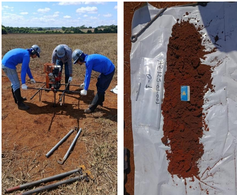
Figure 4 - Auger drilling is being undertaken by two three-man crews. Samples are collected at each 0.5m interval to a nominal depth of five metres at each site. Assaying will be done by ALS, Brazil.
