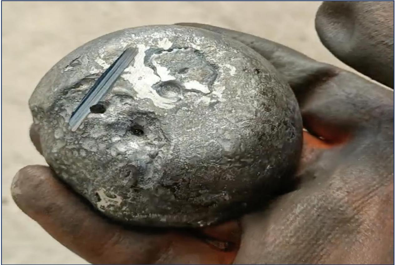
**Figure 9: 100% biochar green pig iron using Buena Vista iron ore.**
