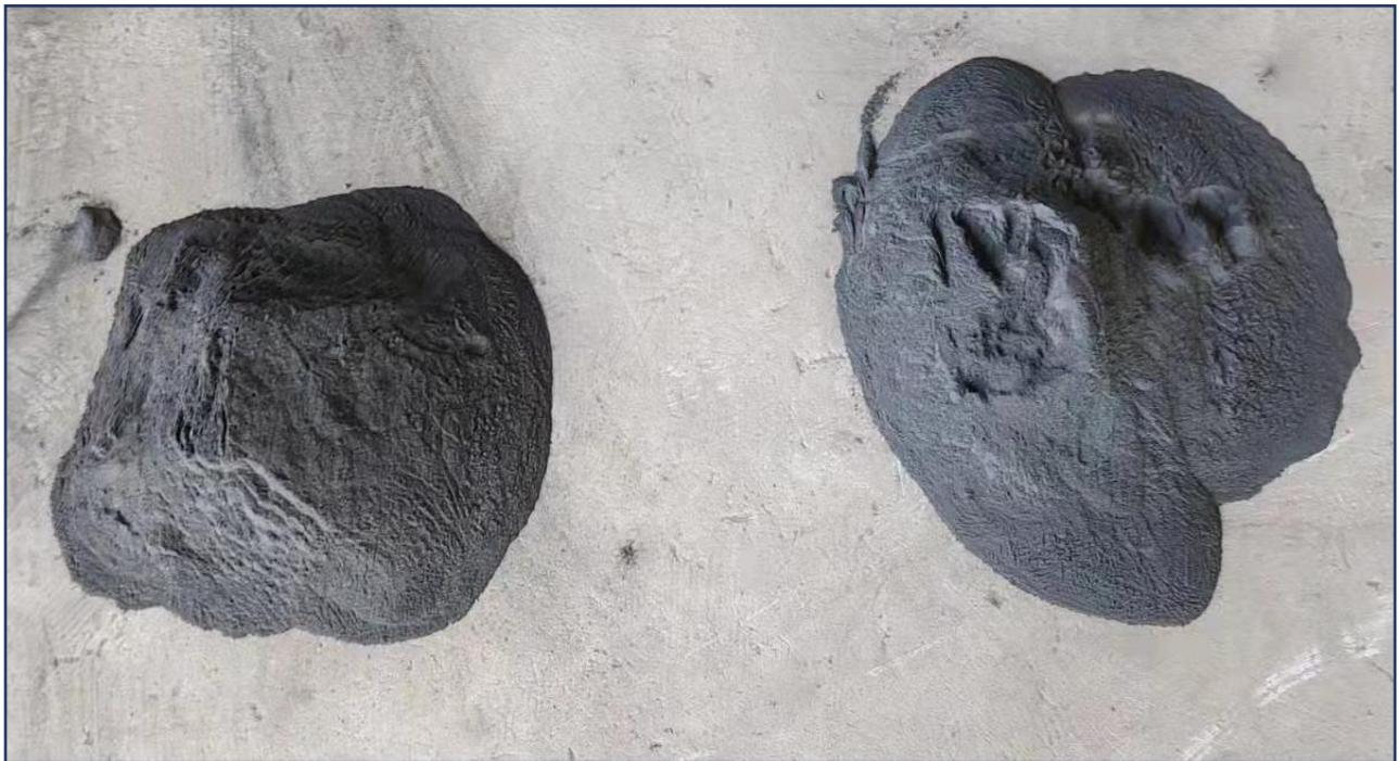
**Figure 6: Buena Vista 63% magnetite iron ore concentrate.**
