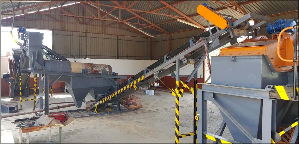
**Photo 6: Plant dewatering screen with trommel and screen feed conveyor**
