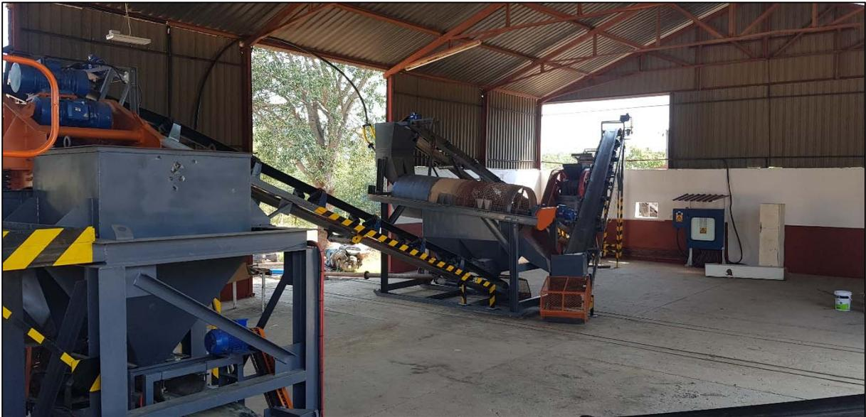
**Photo 7: Plant crusher with oversize return conveyor and trommel**
