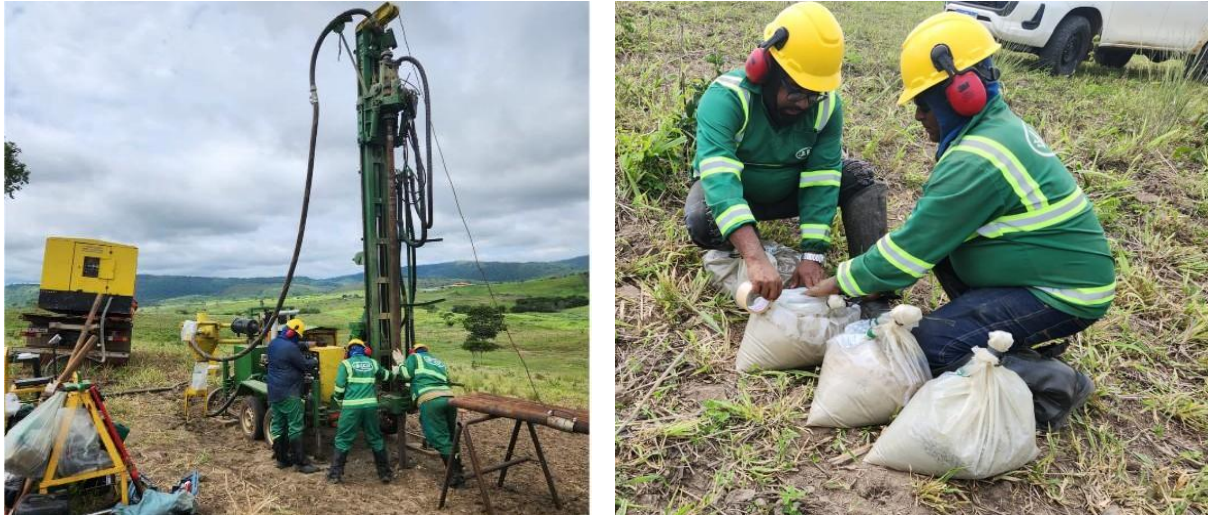
Figure 1 – Left: RC drilling on the Palmares REE Project, at the Feirinha Prospect. Right: Field technicians preparing RC drill samples from Feirinha.
