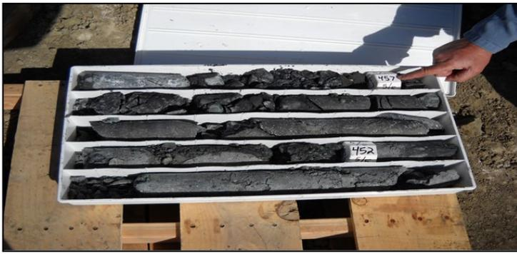
Figure 5: Drill cores showing metasomatic magnetite
